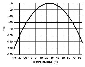
FIGURE 4. RTC CRYSTAL TEMPERATURE DRIFT
