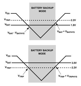
FIGURE 2. BATTERY SWITCHOVER WHEN V<sub>BAT</sub> < V<sub>TRIP</sub> (TOP) AND V<sub>BAT</sub> > V<sub>TRIP</sub> (BOTTOM)
