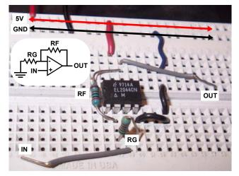
FIGURE 1. BREADBOARDED NON-INVERTING AMPLIFIER CONFIGURATION (A $_V$  = 2)
