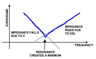
FIGURE 8. IMPEDANCE OF AN ACTUAL CAPACITOR (NON-IDEAL)
