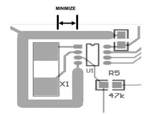
FIGURE 14. SUGGESTED LAYOUT FOR ISL12026 IN REGARDS TO CRYSTAL PLACEMENT
