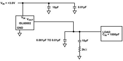
FIGURE 16. VOLTAGE REGULATOR BYPASSING WITH LARGE CAPACITIVE LOAD
