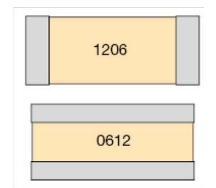
FIGURE 7. EXAMPLE SURFACE MOUNT PACKAGES IN THE 1206 ORIENTATION (TOP) AND THE 0612 ORIENTATION (BOTTOM)
