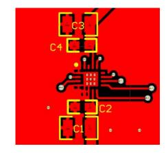
FIGURE 20. LAYOUT OF HIGH SPEED AMPLIFIER HIGHLIGHTING PLACEMENT OF BYPASS CAPACITORS
