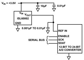
FIGURE 15. VOLTAGE REGULATOR AND ADC BLOCK DIAGRAM
