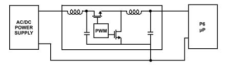
FIGURE 17. SIMPLIFIED BLOCK DIAGRAM OF A DC/DC CONVERTER
