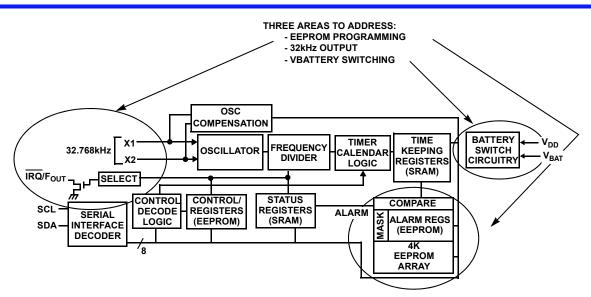
FIGURE 12. BLOCK DIAGRAM OF REAL-TIME CLOCK-CALENDAR WITH EEPROM CIRCUIT
