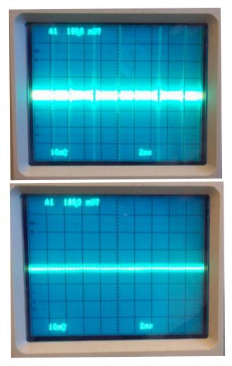
FIGURE 4. OUTPUT OF NON-INVERTING AMPLIFIER SHOWN IN FIGURE 3 WITHOUT BYPASSING (TOP) AND WITH BYPASSING (BOTTOM).
