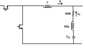
FIGURE 19. SIMPLIFIED DC/DC CONVERTER WITH CAPACITOR PARASITICS
