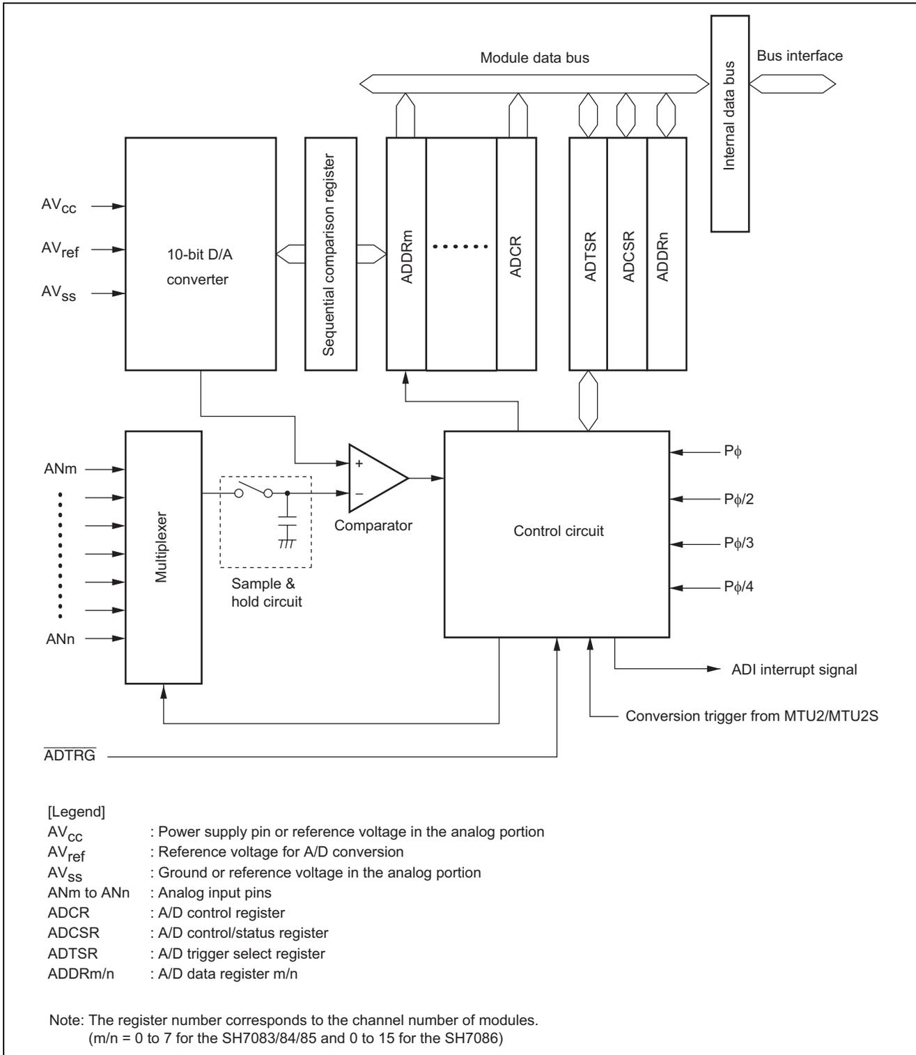
Figure 2 A/D Converter Block Diagram (One Module)
