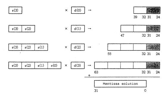
(e) Normalization is performed on the exponent solution and the mantissa solution found in (d), and the result is stored in FPR1 together with the sign bit.
