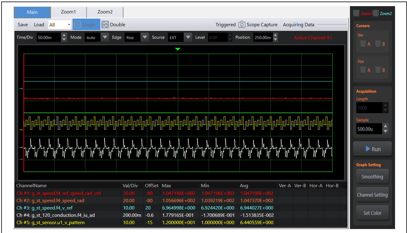
Figure 7-2 Speed control using sensorless 120-degree conducting control
