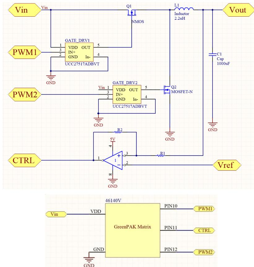
Figure 1. Top level schematic
