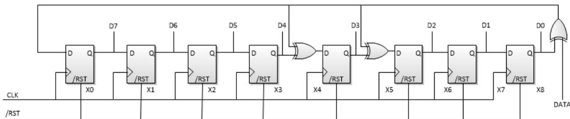
Figure 1. Logic Diagram of 1-Wire CRC Generator Unit
