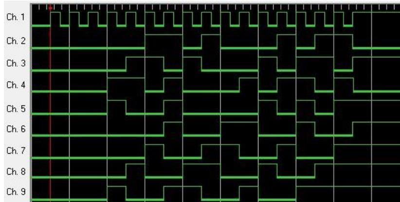
Figure 7. 8-bit 1-wire CRC error code output
