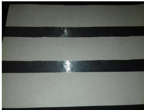
Figure 2. Resistive touch sensor built with metal foil
