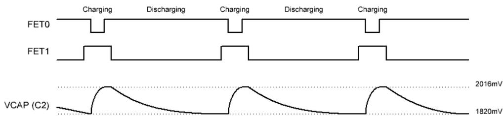
**Figure 3: Timing Diagram**
