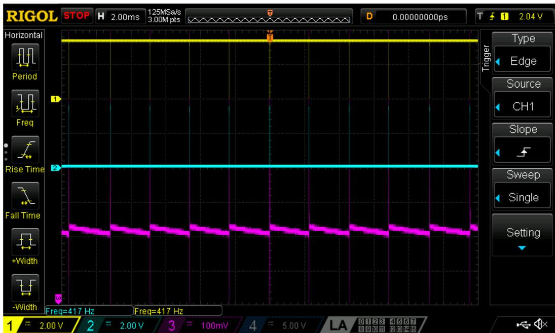
Figure 7: Operation at I\_LOAD = 50  $\mu$ A
