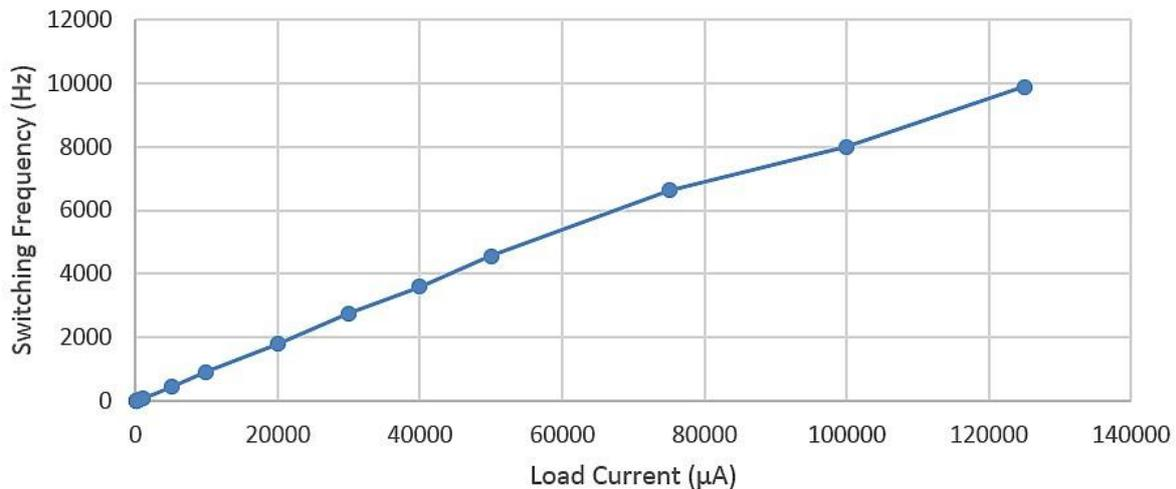
**Figure 10: Load Current vs Switching Frequency, 10 µA to 125 mA**
