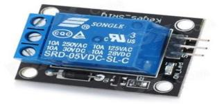
Figure 8. 220V Arduino Relay Board
