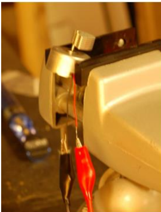
Figure 11: Vibration motor in a vise
