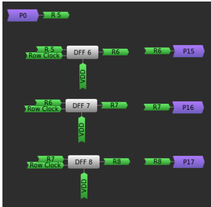
Figure 11. Chaining DFFs R6 to R8 in Matrix1
