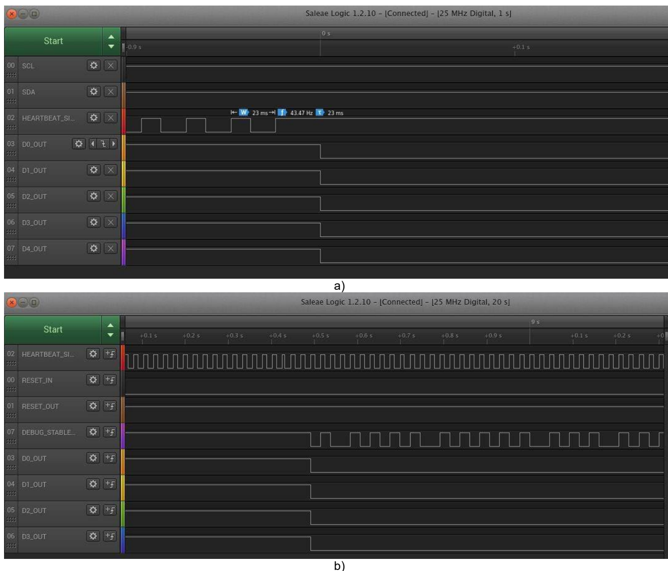
Figure 12. Auto lockout of Output pins when no or fluctuating heartbeat signal (No Signal) (a); Fluctuating Signal(b)
