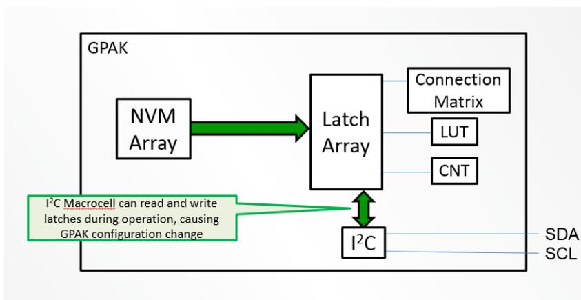
**Figure 3. I<sup>2</sup>C In-System Debug capability**
