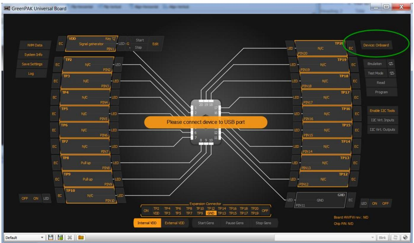
**Figure 4. “Device Onboard” button in GreenPAK Emulation Tool window**
