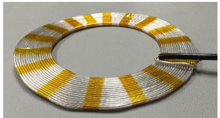
Fig 1b. Example search coil
