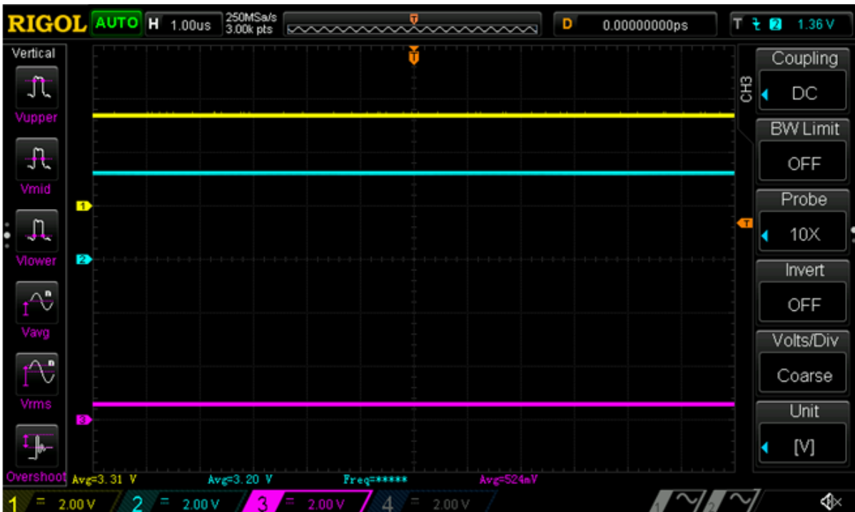
Figure 6: Device functionality then SPI code 192 at VDD 3.3V
