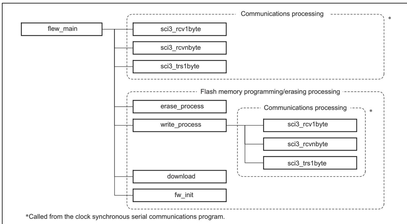
**Figure 18 Programming/Erasing Procedure Program**
