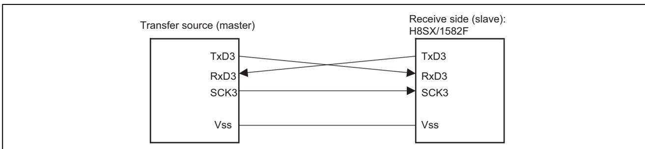
Figure 2 Wiring for Clock Synchronous Communications
