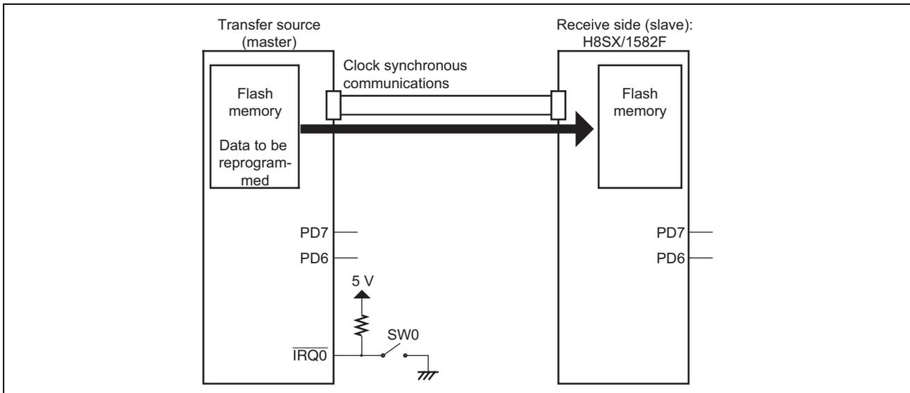
Figure 1 Sample Configuration for On-Board Reprogramming
