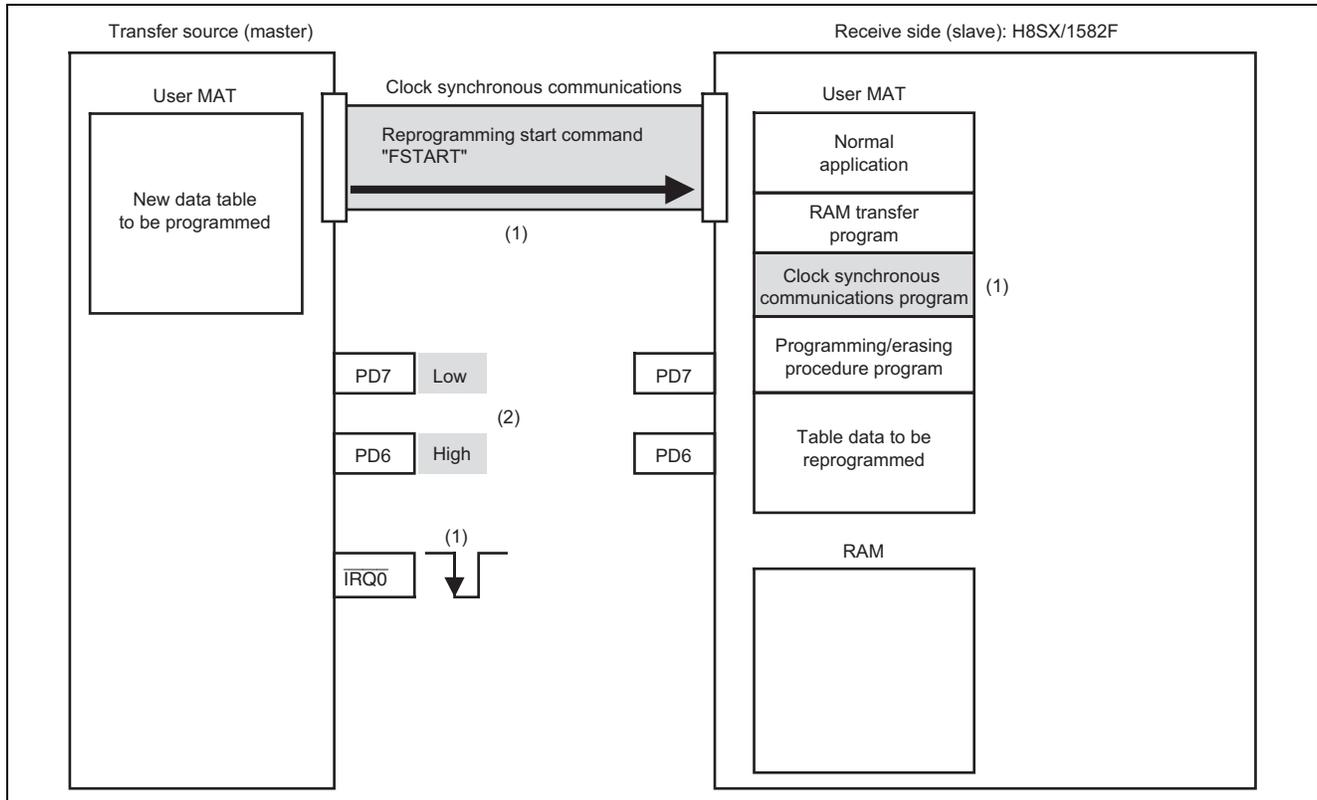
Figure 7 Preparation of On-Board Reprogramming
