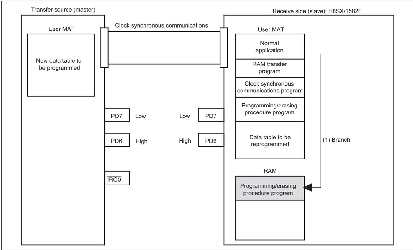
**Figure 9 Activation of Programming/Erasing Procedure Program**
