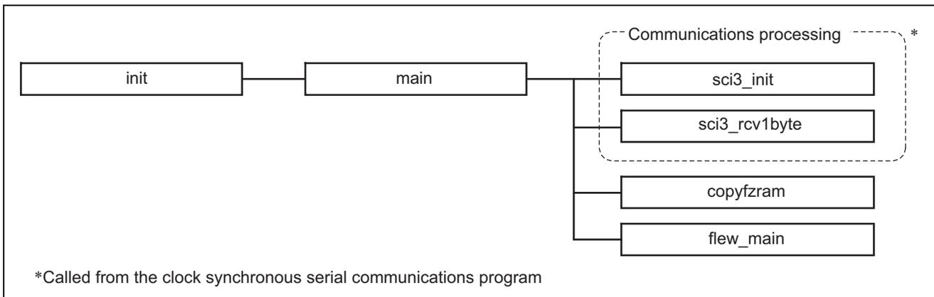
**Figure 17 Normal Program on the Slave Side**
