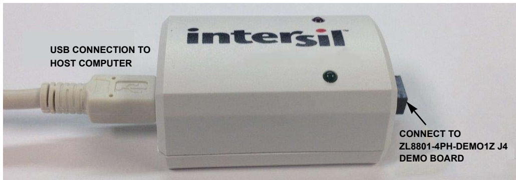
FIGURE 13. USB TO PMBus DONGLE
