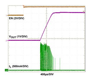
FIGURE 3. SOFT-START (V<sub>IN</sub> = 4V, V<sub>OUT</sub> = 3.3V, NO LOAD)
