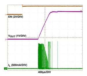
FIGURE 2. SOFT-START (V<sub>IN</sub> = 3V, V<sub>OUT</sub> = 3.3V, NO LOAD)
