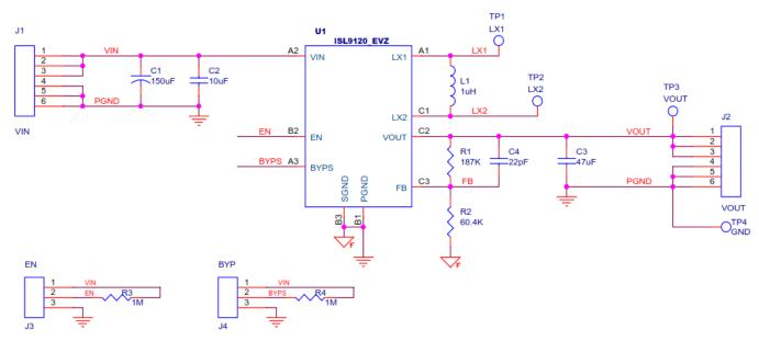
FIGURE 5. ISL9120IIA-EVZ EVALUATION BOARD SCHEMATIC
