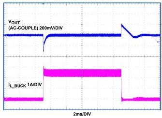
FIGURE 17. LOAD TRANSIENT RESPONSE 0A<->2.5A, VIN = 12V
