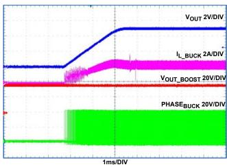
FIGURE 25. SOFT-START WITH  $2\Omega$  LOAD (V<sub>IN</sub> = 36V)
