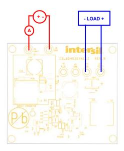
FIGURE 3. ISL85403EVAL1Z BOARD SETUP
