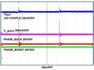
FIGURE 14. OUTPUT RIPPLE AT 0A LOAD (VIN = 36V)
