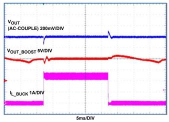
FIGURE 16. LOAD TRANSIENT RESPONSE 0A<->2.5A, V<sub>IN</sub> = 5V
