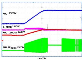
FIGURE 22. SOFT-START AT 0A LOAD ( $V_{IN} = 5V$ )
