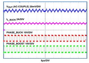
FIGURE 8. OUTPUT RIPPLE AT OA LOAD (V<sub>IN</sub> = 5V)
