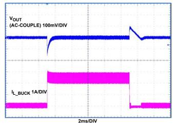
FIGURE 18. LOAD TRANSIENT RESPONSE 0A <-> 2.5A,  $V_{IN} = 24V$
