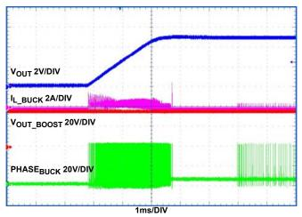
FIGURE 24. SOFT-START AT OA LOAD (V<sub>IN</sub> = 36V)
