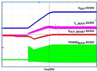
FIGURE 23. SOFT-START WITH  $2\Omega$  LOAD ( $V_{IN} = 5V$ )
