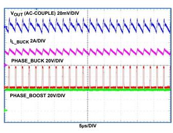
FIGURE 15. OUTPUT RIPPLE AT 2.5A LOAD ( $V_{IN} = 36V$ )
