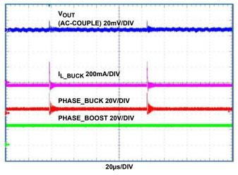
FIGURE 12. OUTPUT RIPPLE AT 0A LOAD (VIN = 24V)
