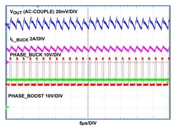
FIGURE 13. OUTPUT RIPPLE AT 2.5A LOAD ( $V_{IN} = 24V$ )
