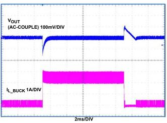
FIGURE 19. LOAD TRANSIENT RESPONSE 0A <-> 2.5A,  $V_{IN} = 36V$
