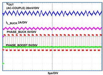
FIGURE 10. OUTPUT RIPPLE AT 0A LOAD ( $V_{IN} = 12V$ )
