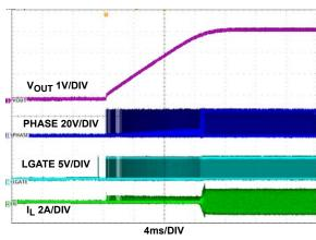
FIGURE 18. CCM START-UP WAVEFORMS:  $V_{OUT}$ , PHASE, LGATE,  $I_L$ ,  $I_D = 0.04$
