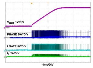
FIGURE 19. DCM START-UP WAVEFORMS:  $V_{OUT}$ , PHASE, LGATE,  $I_{L}$ ,  $I_{0} = 0$ A
