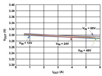
FIGURE 14. CCM LOAD REGULATION
