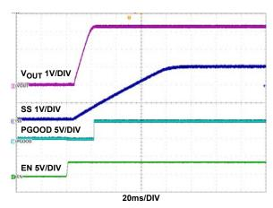
FIGURE 20. CCM START-UP WAVEFORMS:  $V_{OUT}$ , SS, PGOOD, EN,  $I_{O} = 0A$
