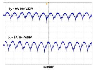
FIGURE 16. OUTPUT RIPPLE, MODE = CCM
