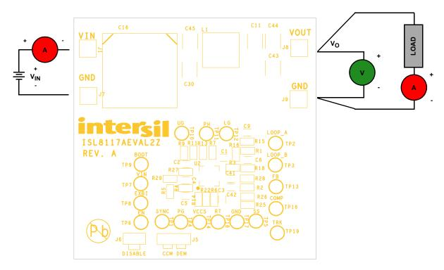
FIGURE 3. PROPER TEST SETUP
