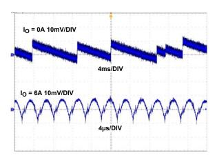
FIGURE 17. OUTPUT RIPPLE, MODE = DEM
