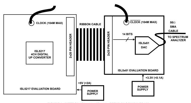
FIGURE 2. INTERSIL ISL5x61 + ISL5217 SETUP BLOCK DIAGRAM
