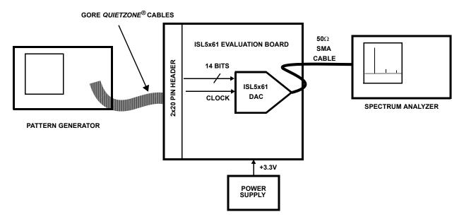
FIGURE 1. INTERSIL ISL5x61 EVALUATION SYSTEM SETUP BLOCK DIAGRAM
