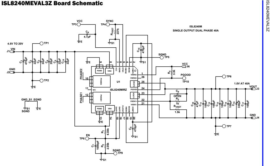
FIGURE 2. ISL8240MEVAL3Z BOARD SCHEMATIC
