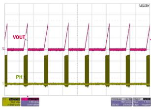
FIGURE 7. OVERCURRENT PROTECTION (VO = 5V, LOAD = 40A)
