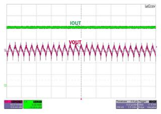
FIGURE 6. OUTPUT RIPPLE (VO = 5V, LOAD = 25A)
