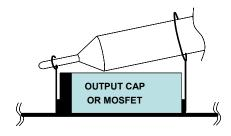
FIGURE 3. OSCILLOSCOPE PROBE SET-UP
