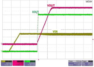
FIGURE 8. SOFT-START AT FULL LOAD
