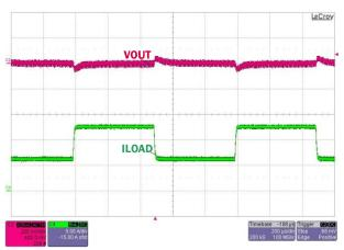
FIGURE 9. LOAD TRANSIENT (25% TO 50% AT  $2A/\mu s$ )
