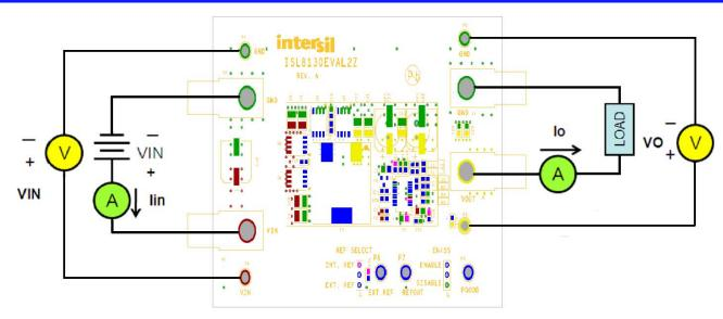
FIGURE 2. ISL8130EVAL2Z TEST SET-UP
