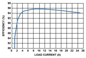
FIGURE 4. EFFICIENCY vs LOAD CURRENT
