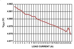
FIGURE 5. LOAD REGULATION, (VIN = 12V, IMAX = 25A)
