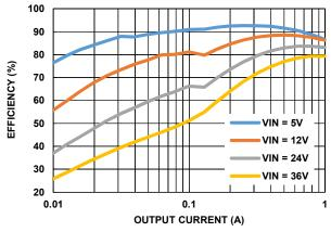
FIGURE 17. EFFICIENCY, PFM (ISL85410EVAL1Z, V<sub>OUT</sub> = 3.3V)
