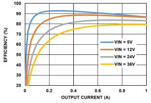
FIGURE 18. EFFICIENCY, PWM (ISL85410EVAL1Z, V<sub>OUT</sub> = 3.3V)
