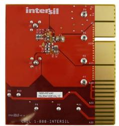
FIGURE 5. BACK OF EVALUATION BOARD ISL854102EVAL1Z
