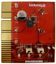
FIGURE 2. FRONT OF EVALUATION BOARD ISL85410EVAL1Z
