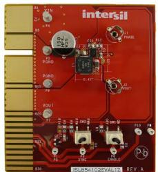
FIGURE 4. FRONT OF EVALUATION BOARD ISL854102EVAL1Z
