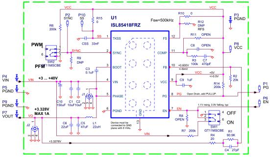
FIGURE 10. ISL85418EVAL1Z SCHEMATIC
