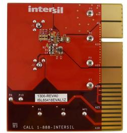
FIGURE 7. BACK OF EVALUATION BOARD ISL85418EVAL1Z
