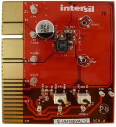
FIGURE 6. FRONT OF EVALUATION BOARD ISL85418EVAL1Z
