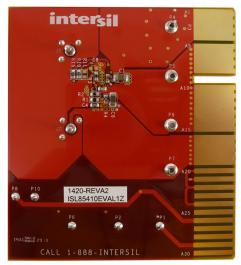
FIGURE 3. BACK OF EVALUATION BOARD ISL85410EVAL1Z
