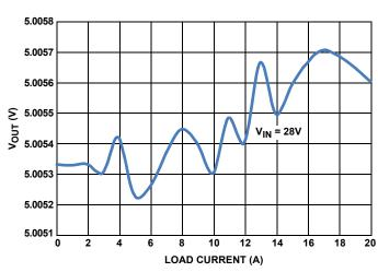
FIGURE 7. V<sub>OUT</sub> LOAD REGULATION AT DEM MODE
