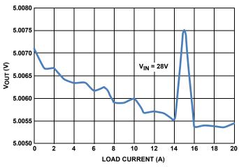
FIGURE 6. V<sub>OUT</sub> LOAD REGULATION AT CCM MODE
