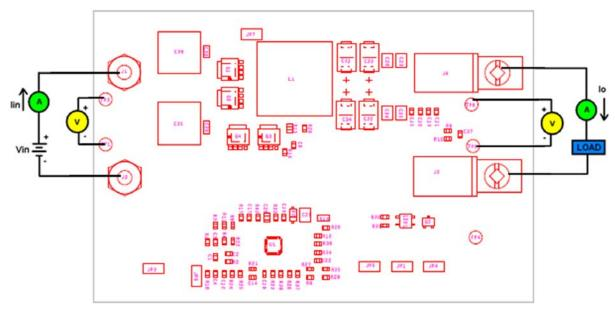
FIGURE 2. ISL8115EVAL2Z TEST SET-UP
