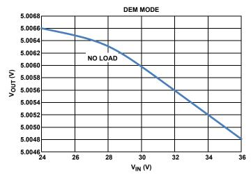
FIGURE 8. LINE REGULATION AT NO LOAD CONDITION
