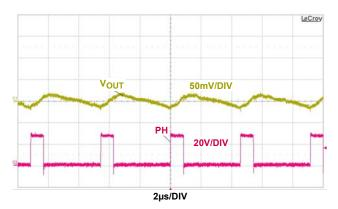
FIGURE 10. OUTPUT VOLTAGE RIPPLE AT 20A LOAD CONDITION
