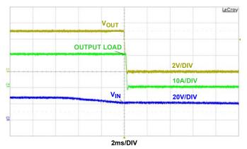
FIGURE 15. SHUTDOWN AT OA LOAD CONDITION
