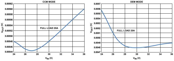
FIGURE 9. LINE REGULATION AT FULL LOAD CONDITION
