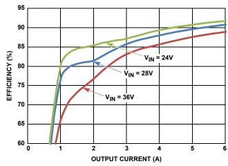
FIGURE 5. EFFICIENCY vs LOAD CURRENT AT DEM MODE
