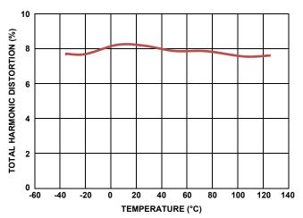
FIGURE 9. VARIATION OF THD WITH AMBIENT TEMPERATURE
