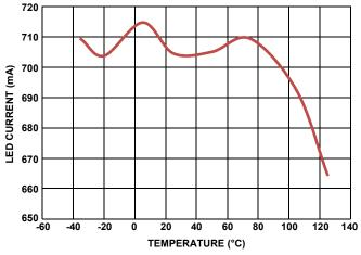
FIGURE 6. VARIATION OF LED CURRENT WITH AMBIENT TEMPERATURE
