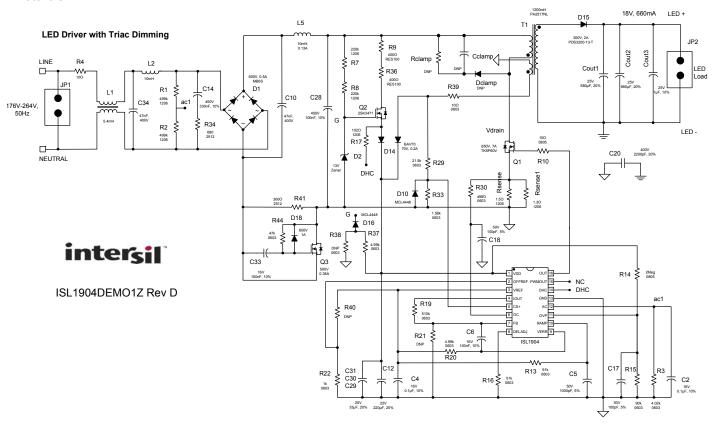
FIGURE 1. ISOLATED FLYBACK CONVERTER APPLICATION SCHEMATIC
