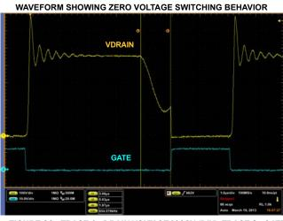
FIGURE 20. TRACE 1 - DRAIN VOLTAGE [100V/DIV); TRACE 2 - GATE [10V/DIV); TDELAY = 1.07µs; PARTIAL ZVS
