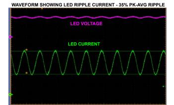
FIGURE 17. TRACE 3 - OUTPUT VOLTAGE [10V/DIV); TRACE 4 - LED CURRENT [200mA/DIV); LED CURRENT RIPPLE: 35% PK-AVG OR 1.35 CREST FACTOR
