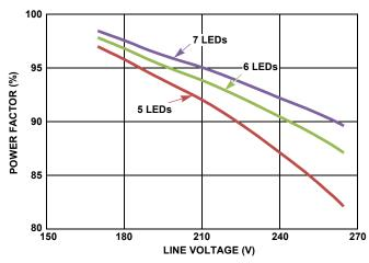
FIGURE 11. POWER FACTOR WITH LINE VOLTAGE AT DIFFERENT LOADS
