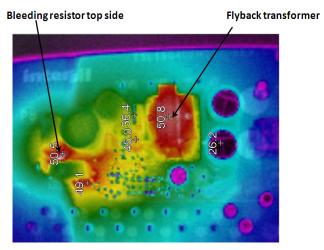
FIGURE 34. TOP SIDE TEMPERATURE SNAPSHOT DURING DEEP DIMMING
