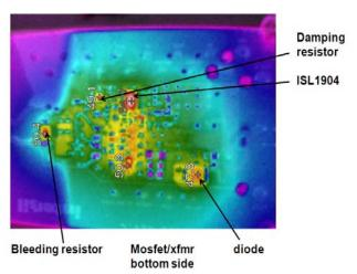
FIGURE 33. BOTTOM SIDE TEMPERATURE SNAPSHOT DURING 100% CONDUCTION AND FULL LOADING
