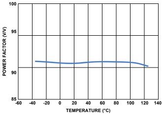
FIGURE 8. VARIATION OF POWER FACTOR WITH AMBIENT TEMPERATURE
