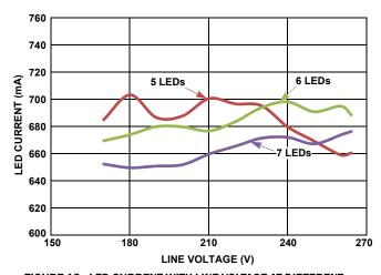
FIGURE 13. LED CURRENT WITH LINE VOLTAGE AT DIFFERENT LOADS
