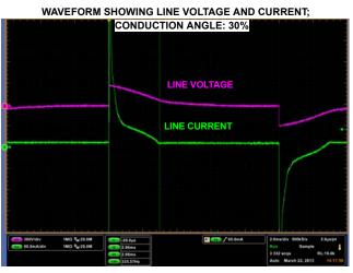
FIGURE 26. TRACE 3 - LINE VOLTAGE [300V/DIV); TRACE 4 - LINE CURRENT [80mA/DIV); 30% CONDUCTION ANGLE
