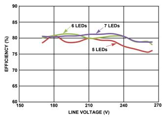
FIGURE 10. EFFICIENCY WITH LINE VOLTAGE AT DIFFERENT LOADS
