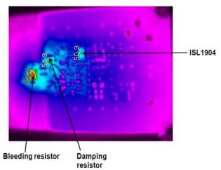
FIGURE 35. BOTTOM SIDE TEMPERATURE SNAPSHOT DURING DEEP DIMMING
