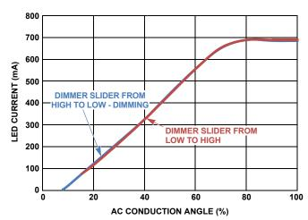
FIGURE 22. DIMMING CURVE - RAMPING DOWN AND RAMPING UP
