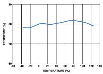
FIGURE 7. VARIATION OF EFFICIENCY WITH AMBIENT TEMPERATURE
