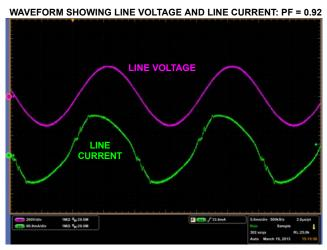
FIGURE 14. TRACE 3 - INPUT VOLTAGE [200V/DIV); TRACE 4 - INPUT CURRENT [60mA/DIV)
