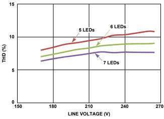
FIGURE 12. THD WITH LINE VOLTAGE AT DIFFERENT LOADS
