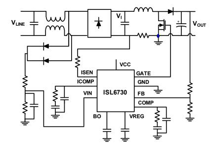
FIGURE 1. SIMPLIFIED SCHEMATIC
