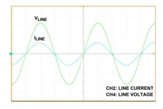
FIGURE 10. WAVEFORMS OF LINE CURRENT AND VOLTAGE (230V/96W)
