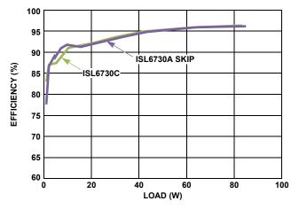
FIGURE 5. HIGH LINE EFFICIENCY vs LOAD
