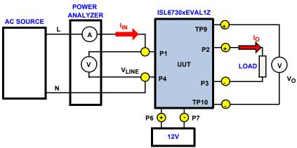
FIGURE 3. TEST SETUP
