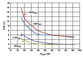
FIGURE 7. THD vs LINE VOLTAGE
