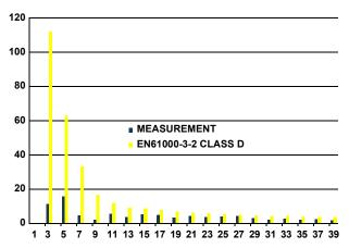
FIGURE 11. HARMONIC CURRENT OF LINE CURRENTS (230V/96W)
