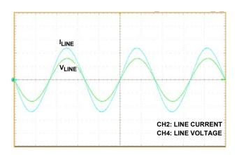
FIGURE 8. WAVEFORMS OF LINE CURRENT AND VOLTAGE (115V/96W)
