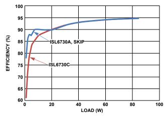
FIGURE 4. LOW LINE EFFICIENCY vs LOAD
