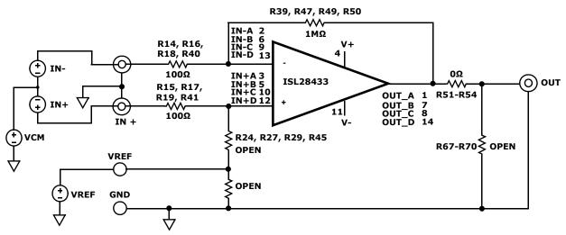
FIGURE 2. BASIC DIFFERENTIAL AMPLIFIER CONFIGURATION
