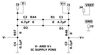
FIGURE 1. POWER SUPPLY CIRCUIT
