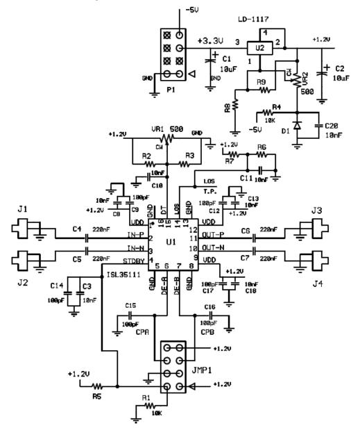
FIGURE 5. ISL35111 EVALUATION BOARD SCHEMATIC
