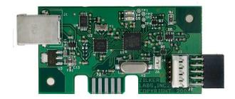
Figure 1. USB to SMBus Interface
