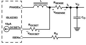
FIGURE 1. RESISTOR CURRENT SENSE CIRCUIT
