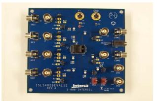
FIGURE 1. ISL54059EVAL1Z THROUGH ISL54064EVAL1Z EVALUATION BOARD
