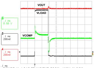
FIGURE 10. LOAD TRANSIENT: FCCM = HIGH, IN CCM BEFORE 250mΩ LOAD-STEP
