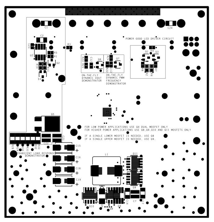
FIGURE 15. PCB BOTTOM SILK SCREEN (MIRRORED)
