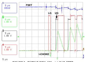
FIGURE 9. EXITING DEM: 250m LOAD-STEP
