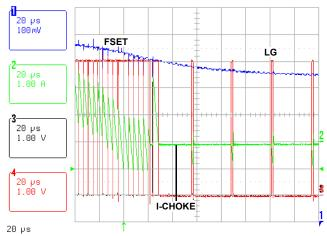
FIGURE 8. ENTERING DEM: 250m  $\Omega$  LOAD-DUMP (UG TOO NARROW TO SEE)
