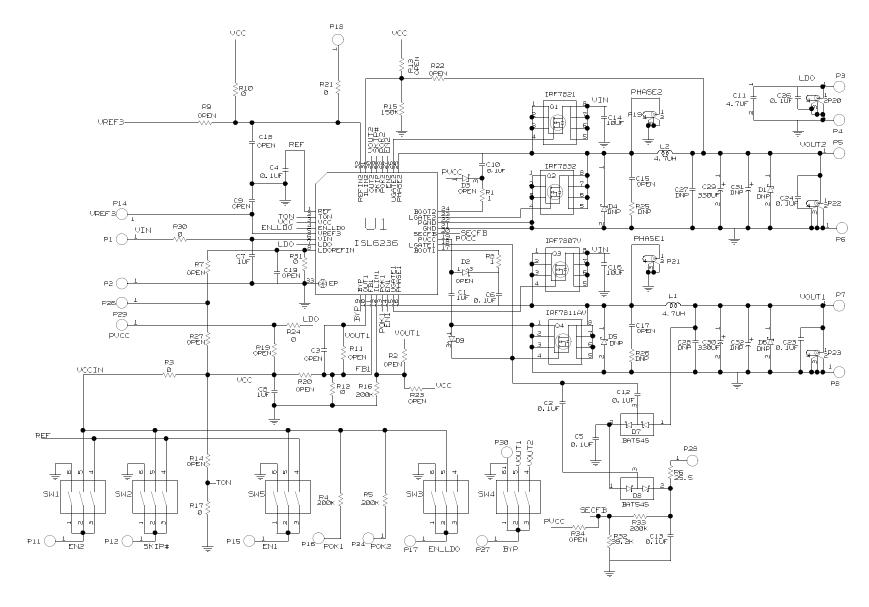
FIGURE 2. ISL6236EVAL1 REV A KIT SCHEMATIC
