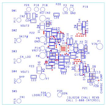
FIGURE 7. BOTTOM COMPONENTS (MIRRORED)
