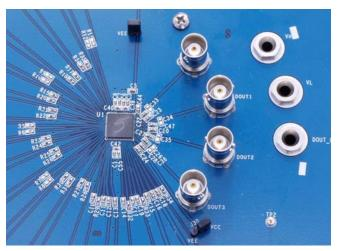
FIGURE 2. DEVICE AREA, ISL55100A/BEVAL3/3Z **EVALUATION BOARD**
