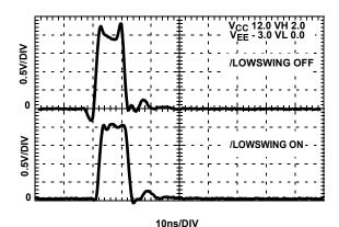
FIGURE 13. LOWSWING CAN BE USEFUL IN SOME APPLICATIONS
