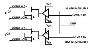
FIGURE 9. WINDOW COMPARATOR USING TTL THRESHOLDS
