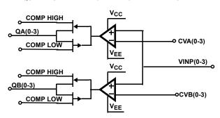
FIGURE 3. DIAGRAM OF ISL55100A/BEVAL3/3Z DRIVERS AND RECEIVERS
