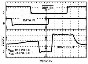
FIGURE 12. DATA AND DRVEN CONTROL OF DRIVER OUT
