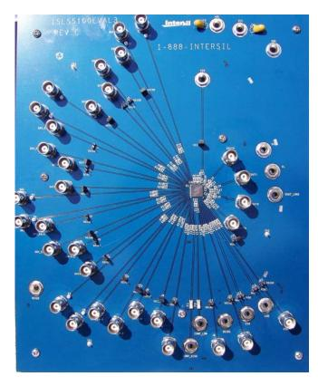
FIGURE 4. ISL55100A/BEVAL3/3Z EVALUATION BOARD
