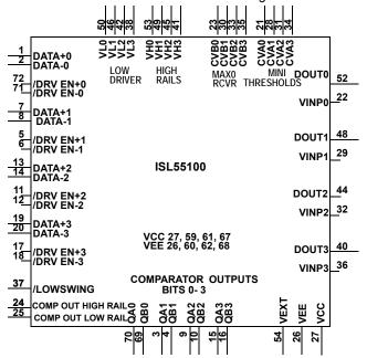
FIGURE 1. FUNCTIONAL ISL55100A/BEVAL3/3Z PINOUT
