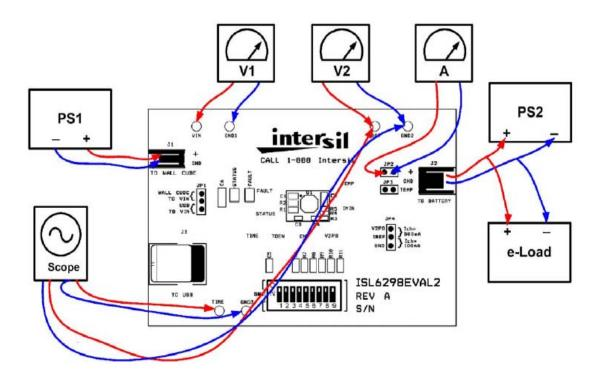
FIGURE 2. CONNECTION OF INSTRUMENTS
