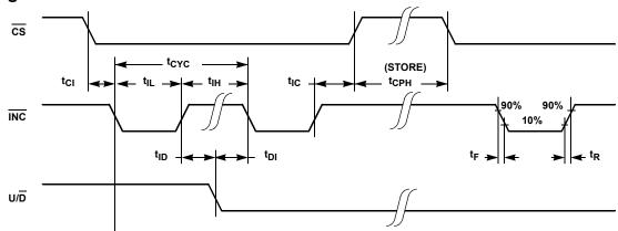
Note:  $\overline{CS}$ ,  $\overline{INC}$ ,  $U/\overline{D}$ ,  $R_H$  and  $R_L$  are used to refer to either  $\overline{CS}_1$  or  $\overline{CS}_2$ , etc.
