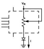
TWO-TERMINAL VARIABLE RESISTOR; VARIABLE CURRENT
