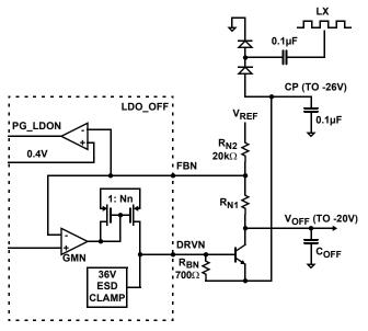
FIGURE 19. VOFF FUNCTIONAL BLOCK DIAGRAM
