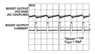
FIGURE 6. BOOST PULSE LOAD TRANSIENT RESPONSE
