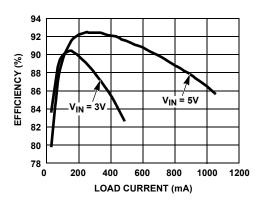
FIGURE 2. BOOST EFFICIENCY AT V<sub>OUT</sub> = 12V (P MODE)
