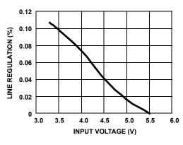
FIGURE 4. BOOST LINE REGULATION vs INPUT VOLTAGE (PI MODE)
