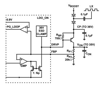
FIGURE 18. VON FUNCTIONAL BLOCK DIAGRAM
