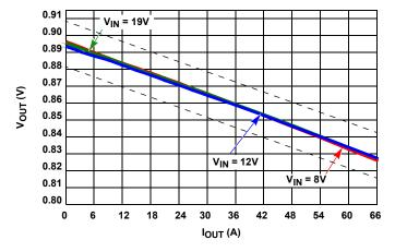
FIGURE 1. LOAD LINE REGULATION
