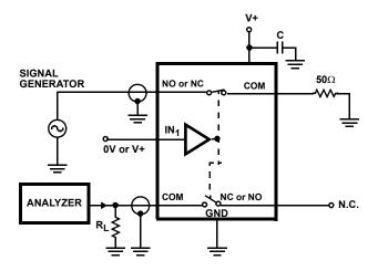
FIGURE 6. CROSSTALK TEST CIRCUIT
