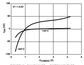
FIGURE 19. ON LEAKAGE vs SWITCH VOLTAGE
