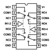
ISL8499 (16 LD 3X3 TQFN, 3X3 QFN) TOP VIEW
