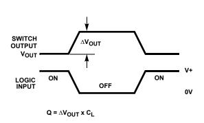
FIGURE 2A. MEASUREMENT POINTS
