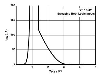
FIGURE 21. SUPPLY CURRENT vs VLOGIC
