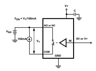
FIGURE 5. ron TEST CIRCUIT
