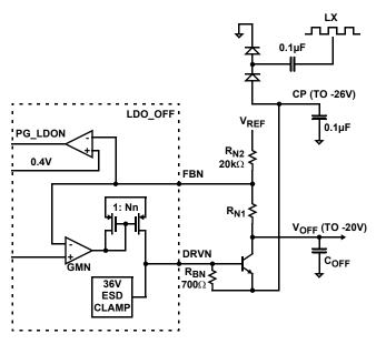
FIGURE 19. VOFF FUNCTIONAL BLOCK DIAGRAM
