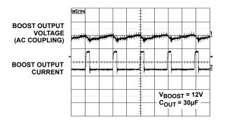
FIGURE 7. BOOST PULSE LOAD TRANSIENT RESPONSE
