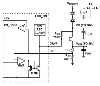
FIGURE 18. VON FUNCTIONAL BLOCK DIAGRAM
