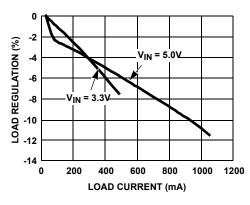
FIGURE 4. BOOST LOAD REGULATION vs LOAD CURRENT (P-MODE)
