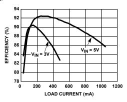
FIGURE 2. BOOST EFFICIENCY AT V<sub>OUT</sub> = 12V (P-MODE)
