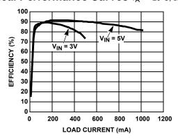
FIGURE 1. BOOST EFFICIENCY AT V<sub>OUT</sub> = 12V (PI-MODE)
