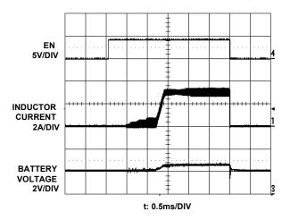
FIGURE 7. CHARGE ENABLE AND SHUTDOWN
