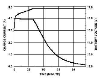
FIGURE 3. BATTERY CHARGE V-I CHARACTERISTICS
