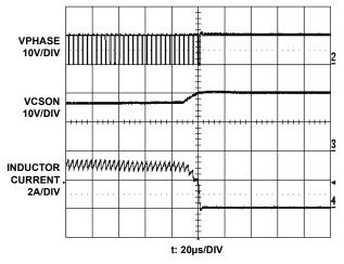
FIGURE 11. BATTERY REMOVAL
