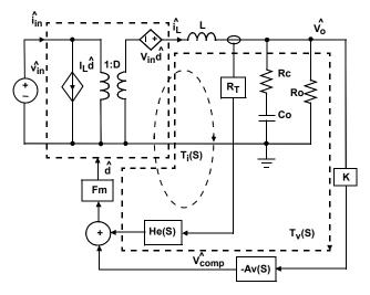
FIGURE 19. SMALL SIGNAL MODEL OF SYNCHRONOUS BUCK REGULATOR
