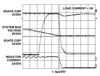
FIGURE 9. AC ADAPTER REMOVAL
