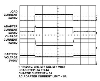
FIGURE 4. LOAD TRANSIENT RESPONSE
