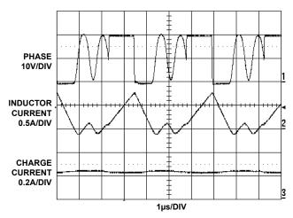
FIGURE 14. SWITCHING WAVEFORMS AT TRICKLE CHARGE MODE
