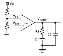
FIGURE 20. TYPE II COMPENSATOR
