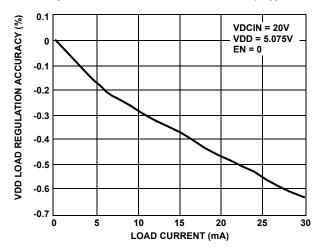
FIGURE 1. VDD LOAD REGULATION
