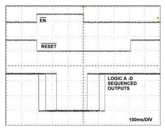
FIGURE 13. ISL6125 LOGIC OUTPUTS SEQUENCED ON AND OFF AND RESET RELATIONSHIP
