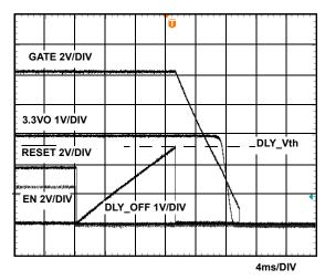
FIGURE 12. ISL6123 SINGLE CHANNEL TURN-OFF
