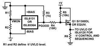
R3 ensures supervisor (ISL6131 or ISL6536A) PGOOD pull-up. R4 and R5 provide Q1 gate bias between 0V and +V to 0V (resistor values suitable for -V = -5V and +V = +3.3V).
