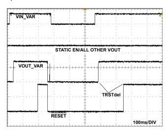
FIGURE 14. ISL6126 UVLO INPUT/OUTPUT INDEPENDENCE AND RESET RELATIONSHIP
