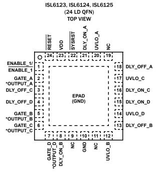
\*OUTPUT\_A, OUTPUT\_B, OUTPUT\_C, OUTPUT\_D ARE UNIQUE TO ISL6125
