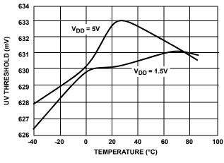
FIGURE 6. UVLO THRESHOLD VOLTAGE
