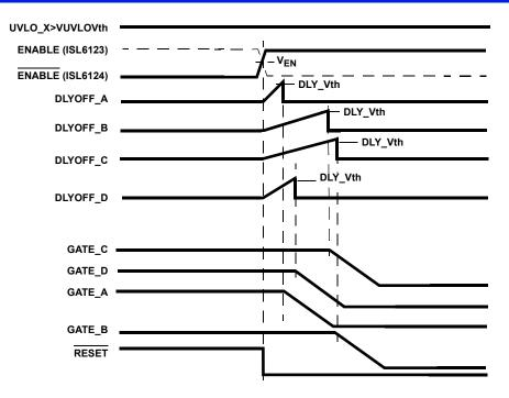
FIGURE 5. ISL6123, ISL6124 TURN-OFF TIMING DIAGRAM
