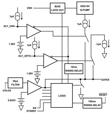
FIGURE 3. ISL6123 BLOCK DIAGRAM (1/4)
