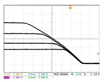
FIGURE 23. OUTPUT VOLTAGE ON HIGH TO LOW TRACKING
