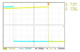
FIGURE 28. CAPACITOR TIMING MISMATCH
