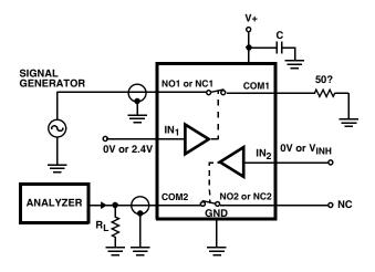
FIGURE 6. CROSSTALK TEST CIRCUIT
