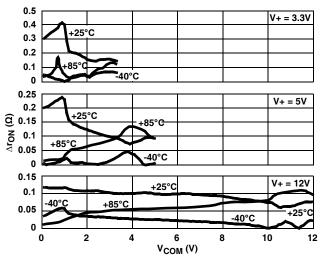
FIGURE 11. ron MATCH vs SWITCH VOLTAGE
