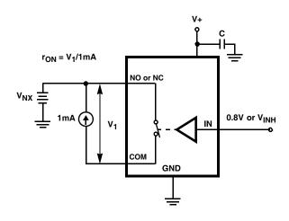
FIGURE 5. ron TEST CIRCUIT
