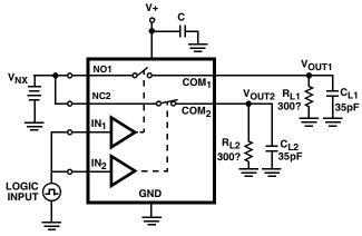
C<sub>L</sub> includes fixture and stray capacitance.
