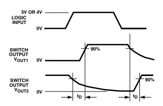
FIGURE 3A. MEASUREMENT POINTS (ISL5122 ONLY)
