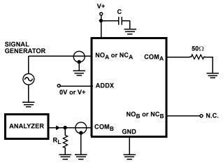
FIGURE 6. CROSSTALK TEST CIRCUIT
