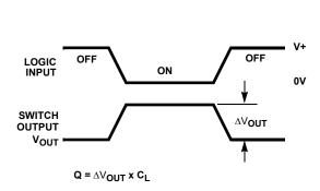
FIGURE 2A. Q MEASUREMENT POINTS
