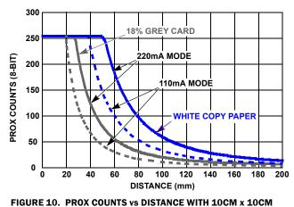
REFLECTOR (USING ISL29028 EVALUATION BOARD)
