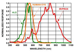
FIGURE 7. ISL29029 SENSITIVITY TO DIFFERENT WAVELENGTHS
