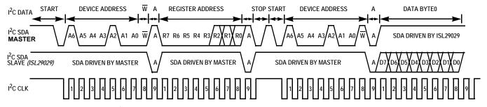
FIGURE 2. I<sup>2</sup>C DRIVER TIMING DIAGRAM FOR MASTER AND SLAVE CONNECTED TO COMMON BUS
