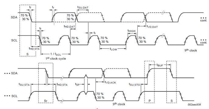
FIGURE 1. I<sup>2</sup>C TIMING DIAGRAM
