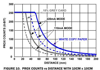
REFLECTOR (USING ISL29028 EVALUATION BOARD)
