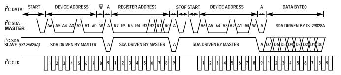
FIGURE 2. 12C DRIVER TIMING DIAGRAM FOR MASTER AND SLAVE CONNECTED TO COMMON BUS
