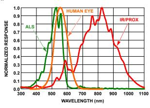
FIGURE 7. ISL29028A SENSITIVITY TO DIFFERENT WAVELENGTHS
