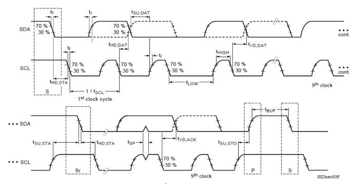
FIGURE 1. I<sup>2</sup>C TIMING DIAGRAM
