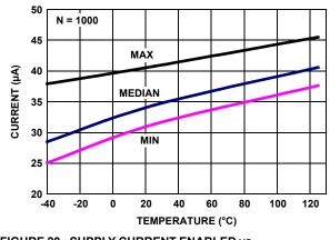
FIGURE 20. SUPPLY CURRENT ENABLED vs TEMPERATURE, V<sub>+</sub>, V<sub>-</sub> = ±2.5V
