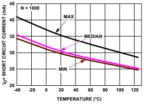
FIGURE 39. I<sub>O</sub>+ SHORT CIRCUIT OUTPUT CURRENT vs TEMPERATURE, V<sub>IN</sub> = -2.55V, R<sub>L</sub> = 10k, V<sub>+</sub>, V<sub>-</sub> =  $\pm 2.5V$
