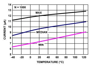
FIGURE 21. SUPPLY CURRENT DISABLED vs TEMPERATURE,  $V_+$ ,  $V_-$  = ±2.5V
