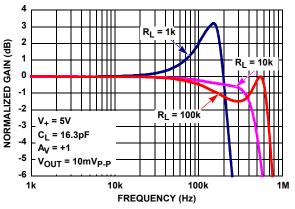
FIGURE 5. GAIN vs FREQUENCY vs RL
