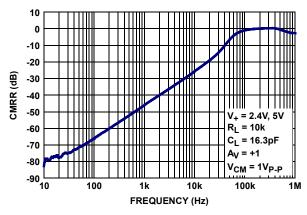
FIGURE 9. CMRR vs FREQUENCY, V<sub>+</sub> = 2.4V AND 5V
