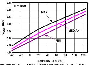
FIGURE 38. V<sub>OUT</sub> LOW vs TEMPERATURE, V<sub>+</sub>, V<sub>-</sub> =  $\pm 2.5V$ , R<sub>L</sub> = 100k
