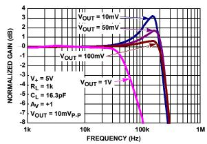
FIGURE 2. GAIN vs FREQUENCY vs V<sub>OUT</sub>, R<sub>L</sub> = 1k
