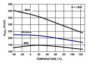
FIGURE 33. A<sub>VOL</sub> vs TEMPERATURE, V<sub>+</sub>, V<sub>-</sub> = ±2.5V, V<sub>O</sub> = -2V TO +2V, R<sub>L</sub> = 100k
