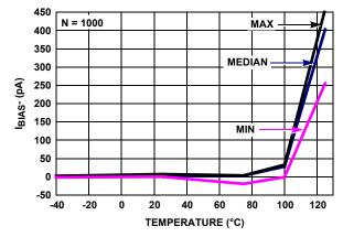
FIGURE 28. IBIAS- vs TEMPERATURE, V+, V\_ = ±1.2V
