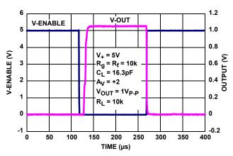
FIGURE 17. ISL28168 ENABLE TO OUTPUT RESPONSE
