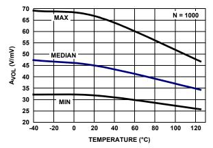
FIGURE 34. A<sub>VOL</sub> vs TEMPERATURE, V<sub>+</sub>, V<sub>-</sub> = ±2.5V, V<sub>O</sub> = -2V TO +2V, R<sub>L</sub> = 1k
