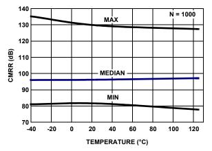
FIGURE 31. CMRR vs TEMPERATURE, V<sub>CM</sub> = -2.5V TO +2.5V, V<sub>+</sub>, V<sub>-</sub> =  $\pm 2.5V$
