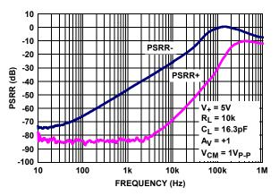
FIGURE 11. PSRR vs FREQUENCY, V+, V = ±1.2V
