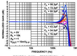
FIGURE 8. GAIN vs FREQUENCY vs CL
