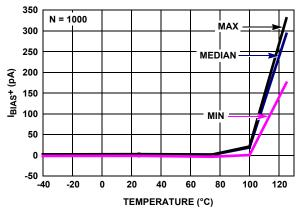
FIGURE 27.  $I_{BIAS}$ + vs TEMPERATURE, V<sub>+</sub>, V<sub>-</sub> = ±1.2V
