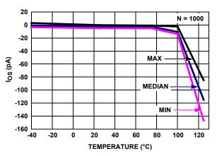
FIGURE 29. IOS vs TEMPERATURE, V+, V\_ = ±2.5
