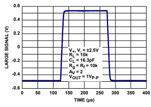
FIGURE 15. LARGE SIGNAL STEP RESPONSE
