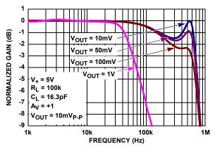
FIGURE 4. GAIN vs FREQUENCY vs V<sub>OUT</sub>, R<sub>L</sub> = 100k
