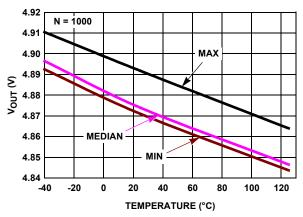
FIGURE 35. V<sub>OUT</sub> HIGH vs TEMPERATURE, V<sub>+</sub>, V<sub>-</sub> = ±2.5V,  $R_L$  = 1k
