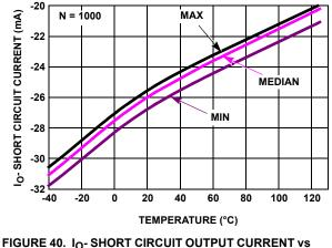
FIGURE 40. I<sub>O</sub>- SHORT CIRCUIT OUTPUT CURRENT vs TEMPERATURE, V<sub>IN</sub> = +2.55V, R<sub>L</sub> = 10k, V<sub>+</sub>, V<sub>-</sub> = ±2.5V
